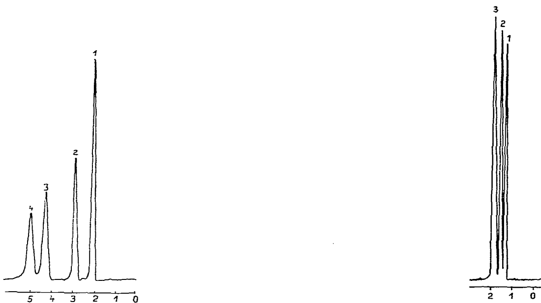
Fig. 6. Separation of C 5 alcohols: tert. -pentanol (1), 2-pentanol (2), 4-methylbutanol-1 (3), pentanol-1 (4). Column as in Fig. 1 at T_c = 110^\circ and F_0 = 24.8 ml/min.
